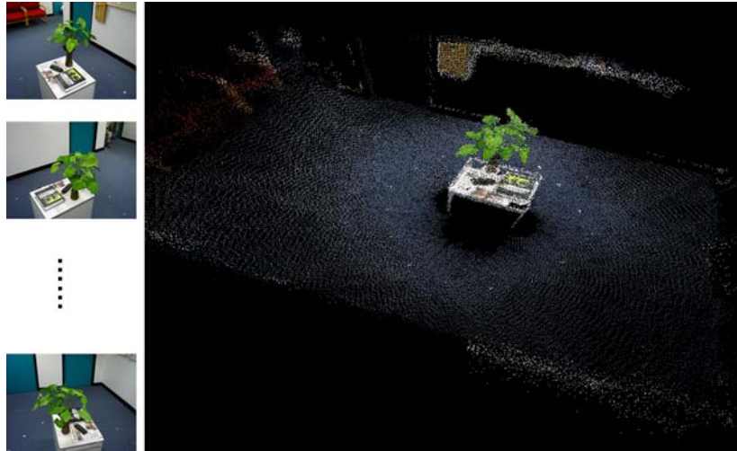
Figure 1. One overview on the right of the reconstructed quasi-dense points for the entire scene from 25 images shown on the left.
